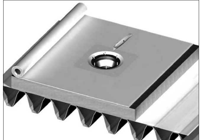
Illustration 10.29 Laying the top layer
