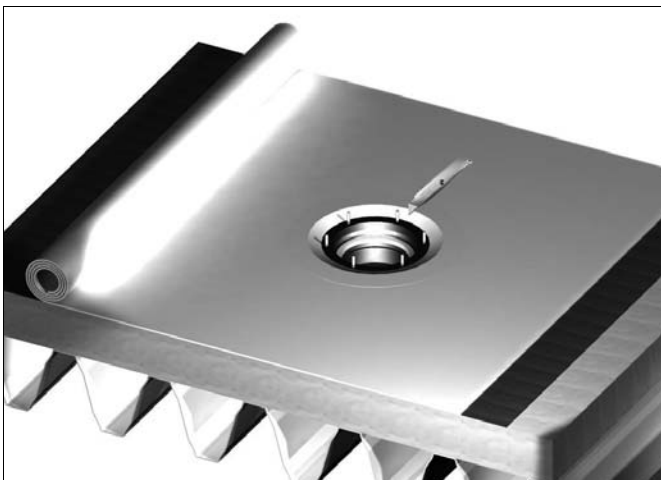
Illustration 10.28 Removing superfluous PVC
