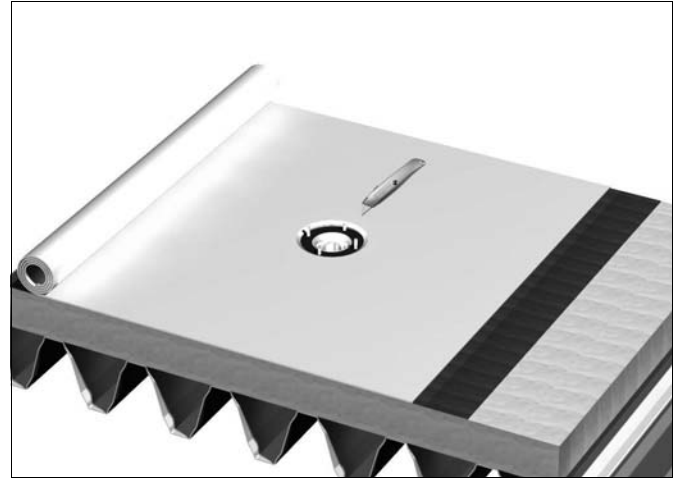
Illustration 10.51 Removing superfluous roofing
