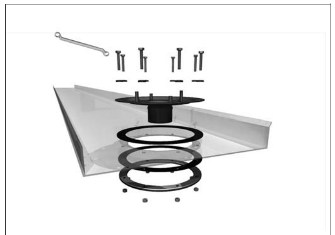
Illustration 10.16 Installing the outlet
