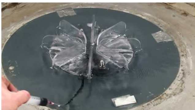
(c) disc with fins, no vortex (ink injected)
