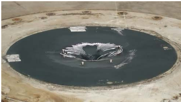
(a) no disc or air baffle, large vortex
