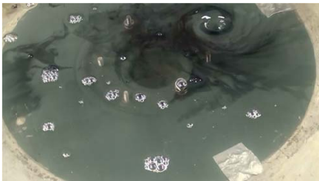
(b) disc, vortex at edge of disc (ink injected)
